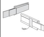
For double glazing in metal frames, minimize the glass/frame allowance, use FS 1/4 Dbl., 3542, and bond glass/ art/FrameSpace package into frame with a bead of silicone glue under frame lip. Apply glue to the frame, assemble frame face up, rest face down overnight to cure.
