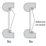
Centering the glass in the frame with the EconoSpace or bonding to the rabbet will result in early adhesive failure.
